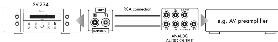
If the input "LINE5" has been selected, the amplifier SV-234 acts like a stereo power amplifier. If you want the amplifier SV-234 to automatically switch on/off every time the HiFi component connected to "LINE5" is switched on/off, the power control cable connections subsequently described must be applied.
