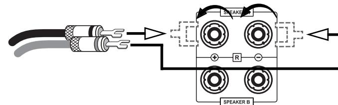
If no connector is to be used, remove approximately 1 cm length of insulation from each end of the speaker wire. Twist the braid in order to avoid short circuits. Turn the fastener on the loudspeaker terminal counterclockwise to loosen it and introduce the bare wire end into the exposed connector hole. Then turn the fastener clockwise so that the wire is firmly clamped. Make sure the connection is pretty tight.
